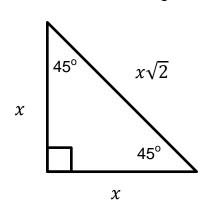
This is an isosceles triangle, so the lengths of the legs are equal.
